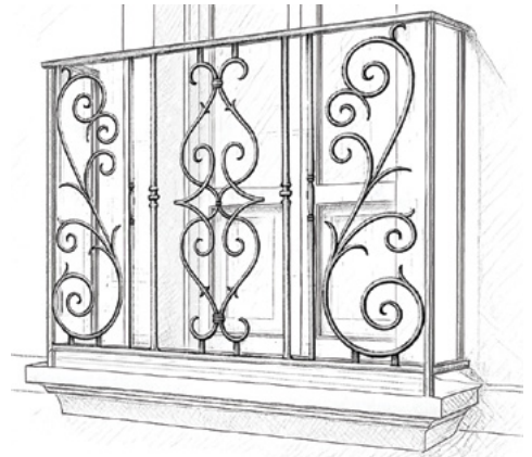
● 539* Malleable Iron 7.8 lbs Cross Section: Scroll – 5/8" x 7/16" Ends – 1/2" x 1/2"
